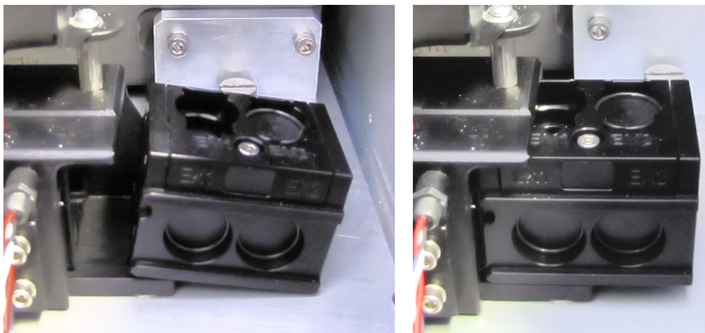
Figure 4-4: Filter cube sliding into the chamber (left) and properly seated (right)
