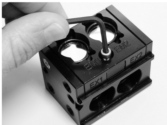
Figure 4-5: Removing the screw located between the EM1 and EM2 positions
